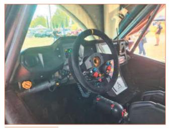
Fig. 3: Equipped dashboard integrating recycled carbon mat © VESO Concept
