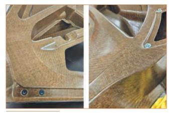
Fig.5: Assembled flax-based door interior © VESO Concept
